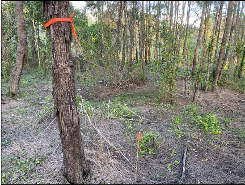
Figure 8 The likely extent of HAT marked at the boundary between salt tolerant and not salt tolerant vegetation in the understory of the swamp she-oak forest.
